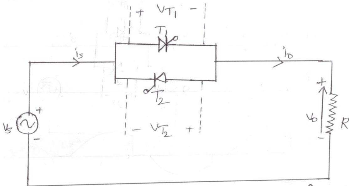
⇒ Thyristors  $T_1$  and  $T_2$  are forward-biased during positive and negative half cycles respectively.
