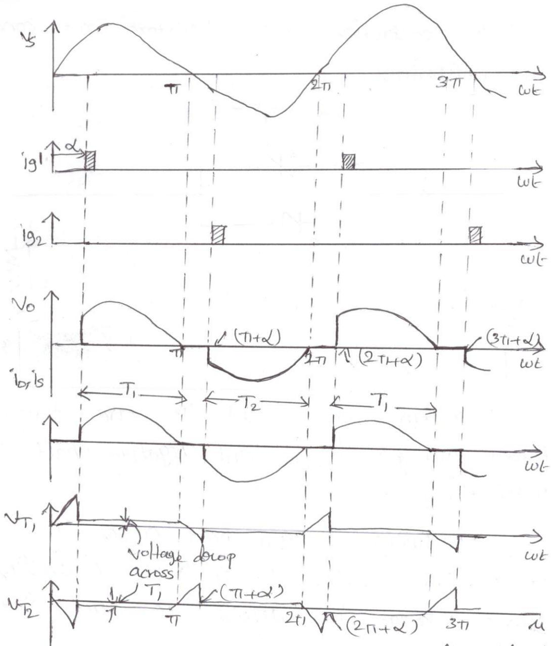
$\Rightarrow$  From zero to  $\alpha$ ,  $T_1$  is forward biased,  $V_{T1} = V_s$ . From  $\alpha$ ,  $T_1$  conducts,  $V_{T1}$  is therefore about  $V$ . After  $\pi$ ,  $T_1$  is reverse biased by source voltage, therefore  $V_{T1} = V_s$  from  $\pi$  to  $\pi + \alpha$ .
