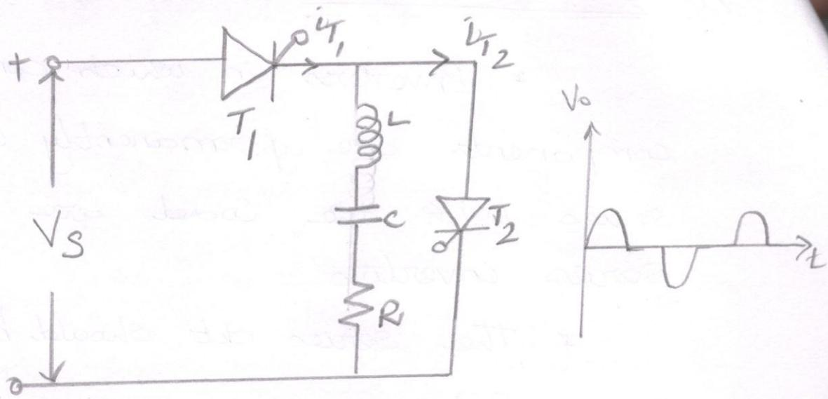
\* When  $T_1$  turned on, with  $T_2$  turned off, current  $i$  starts building up in the RLC ckt.
