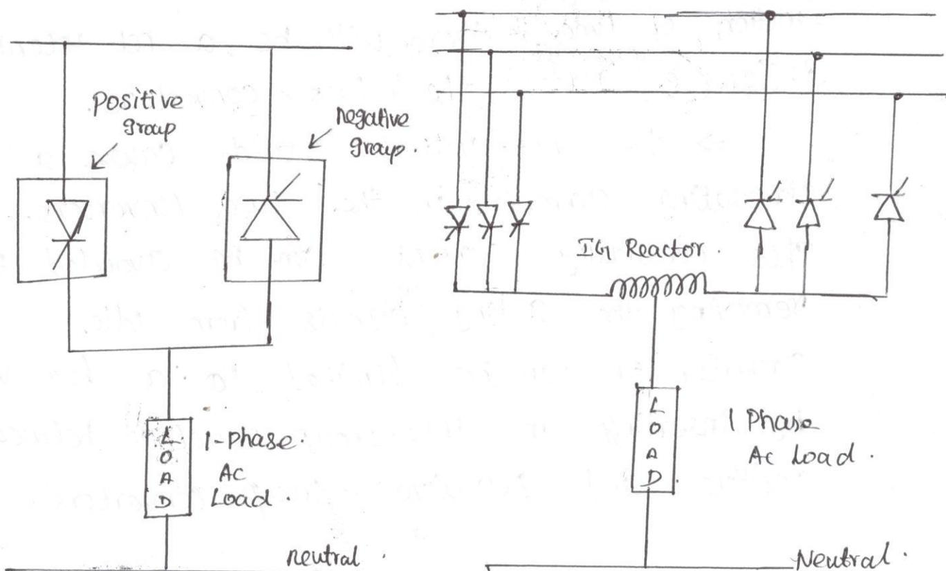
⇒ when output current is positive, positive converter conducts. Under this condition, positive converter acts as a rectifier when output voltage is positive and as an inverter when output voltage is negative.
