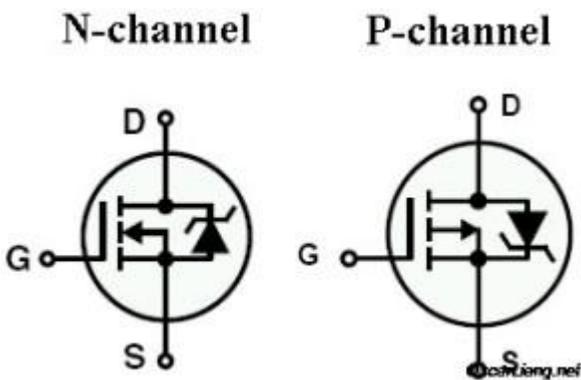
A MOSFET may be thought of as a variable resistor, where the Gate-Source voltage difference can control the Drain-Source Resistance. When there is no applying voltage between the Gate-Source, the Drain-Source resistance is very high, which is almost like a open circuit, so no current may flow through the Drain-Source. When Gate-Source potential difference is applied, the Drain-Source resistance is reduced, and there will be current flowing through Drain-Source, which is now a closed circuit.
