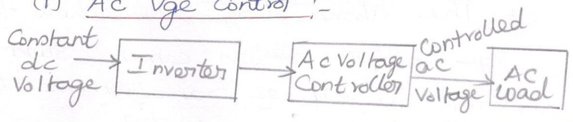
\* An ac vge controller is inserted b/w the o/p terminals of inverter & the load terminals.
