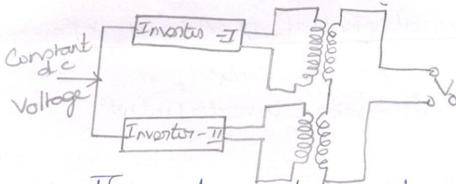
\* The above diag. shows how the o/p vge of two inverters can be summed up with the help of transformers whose o/p vge can be adjusted.
