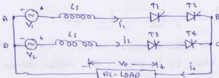
Let us consider the case when  $L_s$  is not present i.e. when the source inductance is zero. Here the source is connected but  $T_1 + T_2$  are fixed at  $\alpha$ .
