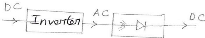
→ dc is first converted to ac by an inverter (dc to ac converter)
