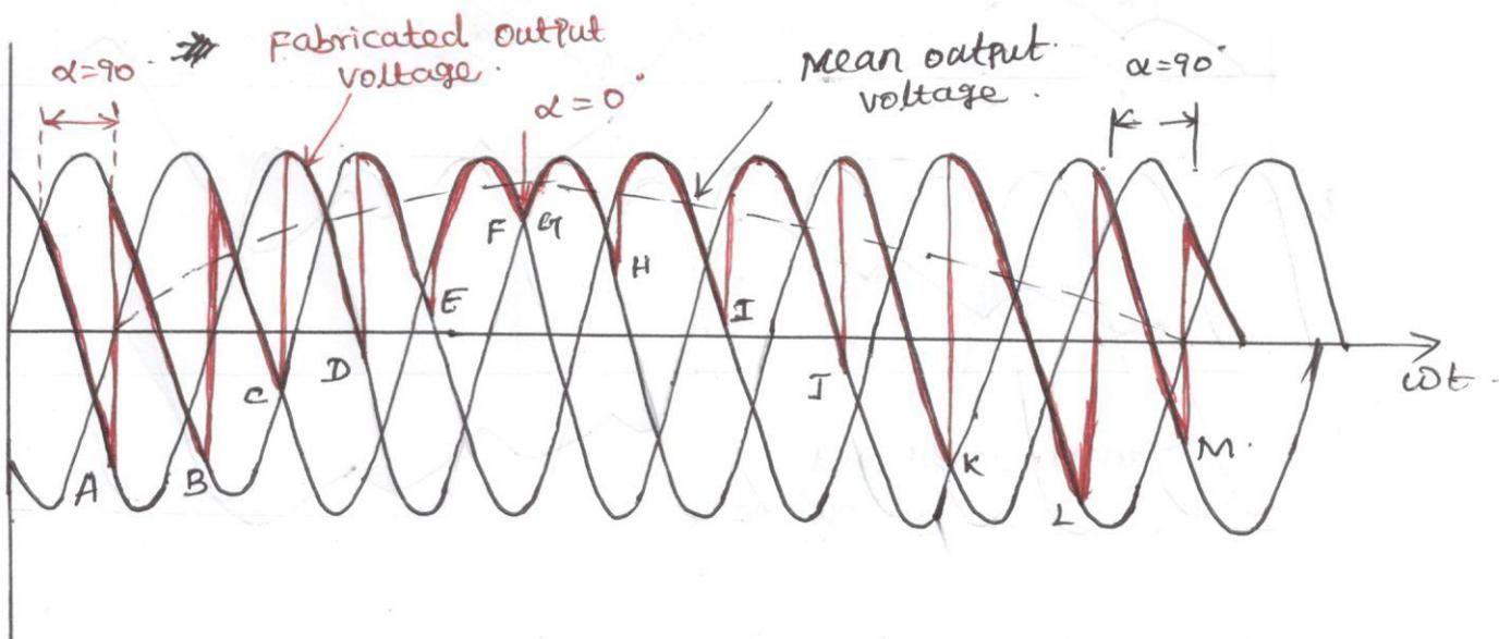
⇒ At A, the mean output voltage is zero as  $\alpha = 90^\circ$ . After point G, a small delay in firing is further introduced progressively at points H, I, J, K, L and M. At M, the firing angle is again  $90^\circ$  and the value of mean output voltage is zero.
