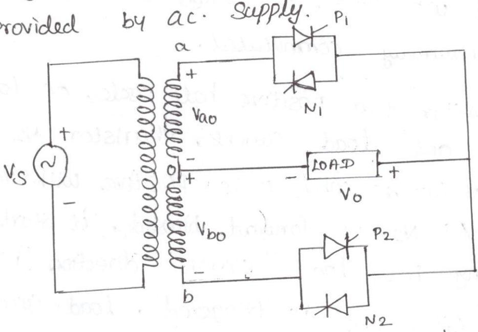
⇒ This type of cycloconverter will be described both for discontinuous as well as continuous load current.
