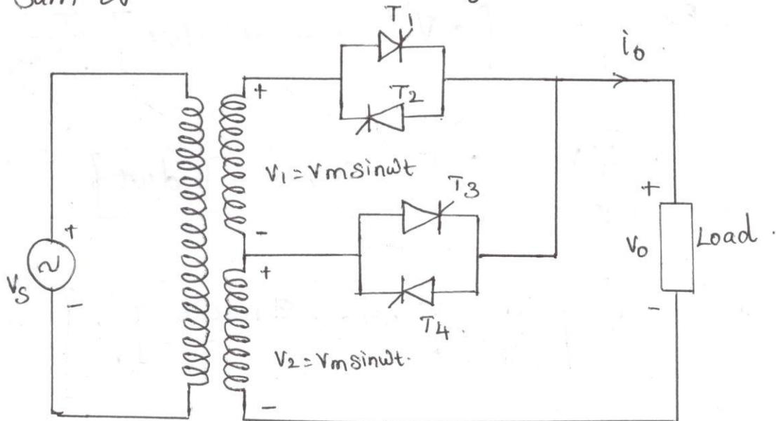
⇒ For obtaining output voltage control from zero to rms value  $V$ , use only thyristor pair  $T_3, T_4$ .
