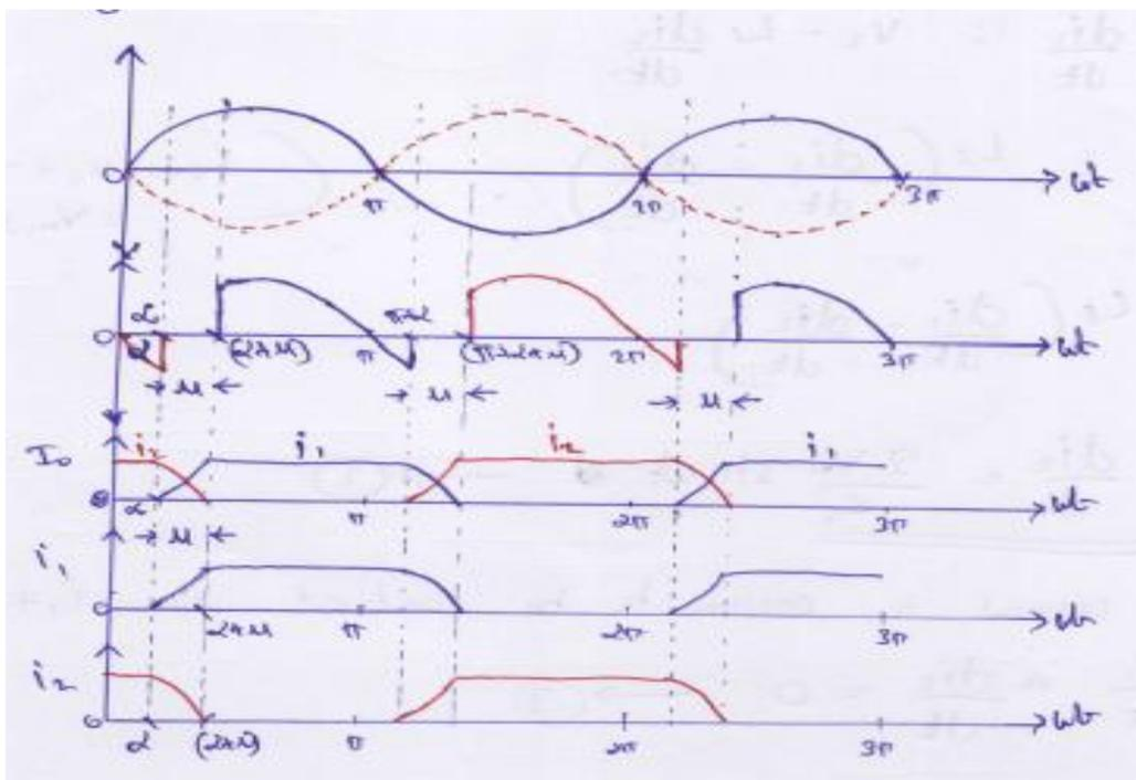
from figure, we can see that,  $V_o$  is 0 for  $\alpha$  to  $\alpha + \mu$
