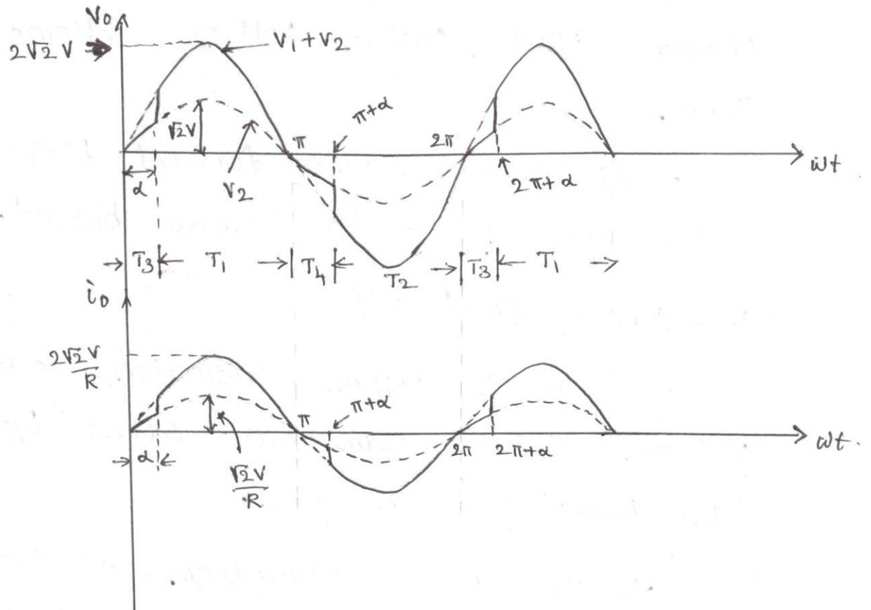
$\Rightarrow$  When both pairs,  $T_1, T_2$  and  $T_3, T_4$  are in operation, then firing angle for  $T_3, T_4$  is always zero whereas firing angle for pair  $T_1, T_2$  is varies from  $180^\circ$  to zero for obtaining output voltage from  $V$  to  $2V$
